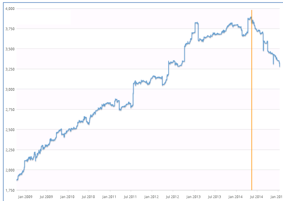
Fig. 1. Example of the development of the number of quality defects after the introduction of incremental quality analysis to a software project. The introduction of the tool is marked by the vertical line.
