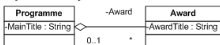
BMF is formulated with different modeling technologies. It was first developed as an entity-relationship diagram which later has been replaced with a UML class diagram. To leverage data exchange by means of XML documents an XML Schema was dynamically generated from the BMF UML class diagram. Furthermore the data model is currently being registered at the Society of Motion Picture and Television Engineers (SMPTE), which requires its own format for data models [SMPTE03,SMPTE01,SMPTE08].
